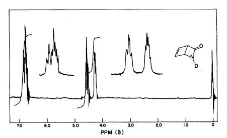
Figure 1. The 60-MHz pmr spectrum of photo-2-pyridone (2a) in CDC13 after  $D_2O$  exchange (Varian T-60). Inserts are expansions at 250 Hz sweep width.
